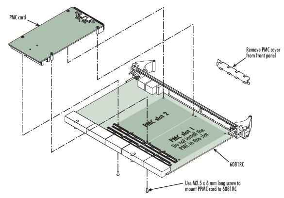
Figure 5. Installing the PMC card
